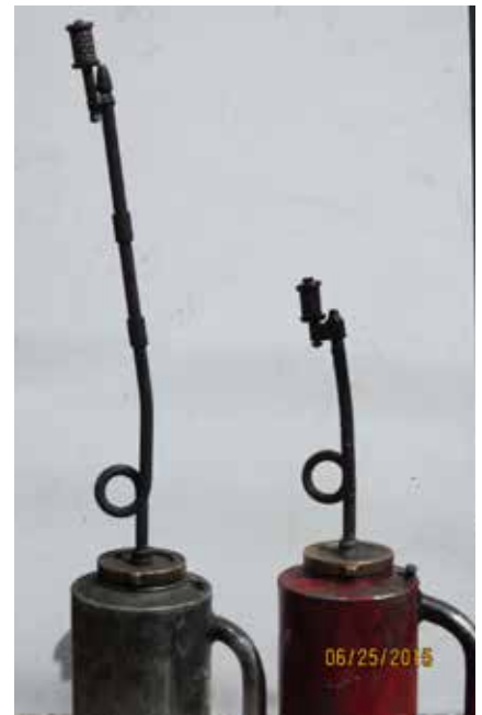
Figure 3: The drip torch on the left has been modified to extend the wand while the drip torch on the right has a standard length wand.
